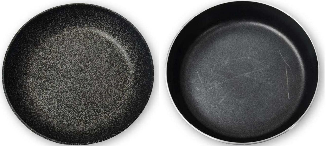
*The demanding CAMUT test shows impressively the difference between the Teflon™ Profile nonstick coating (left) and a conventional PTFE coating (right); © Chemours*
