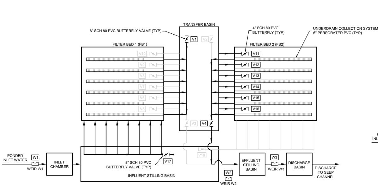
9 SCHEMATIC FLOW THROUGH CELL SYSTEM FLOW WITH CARBON BED 1 IN LEAD POSITION AND CARBON BED 2 IN LAG POSITION
