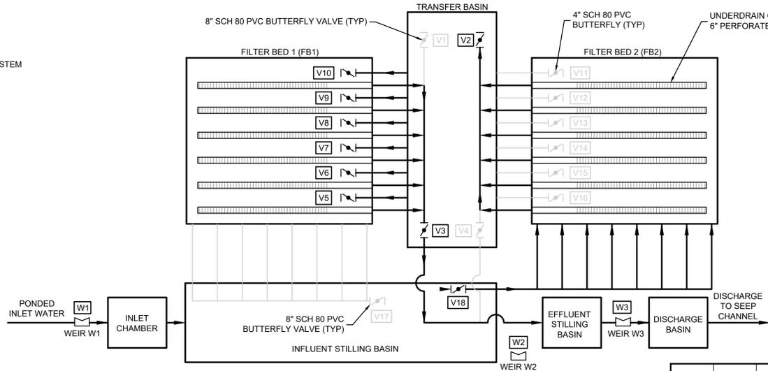
10 SCHEMATIC FLOW THROUGH CELL SYSTEM FLOW WITH CARBON BED 2 IN LEAD POSITION AND CARBON BED 1 IN LAG POSITION
