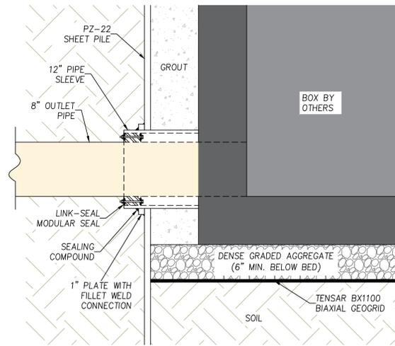
2 LINK-SEAL PIPE THROUGH WALL CONNECTION
