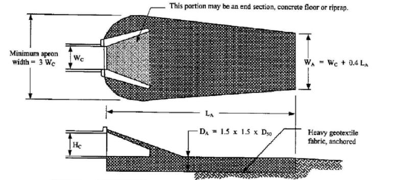
Tailwater > 0.5 H<sub>c</sub> and Assuming Full Culvert Flow (High Tailwater Conditions)
