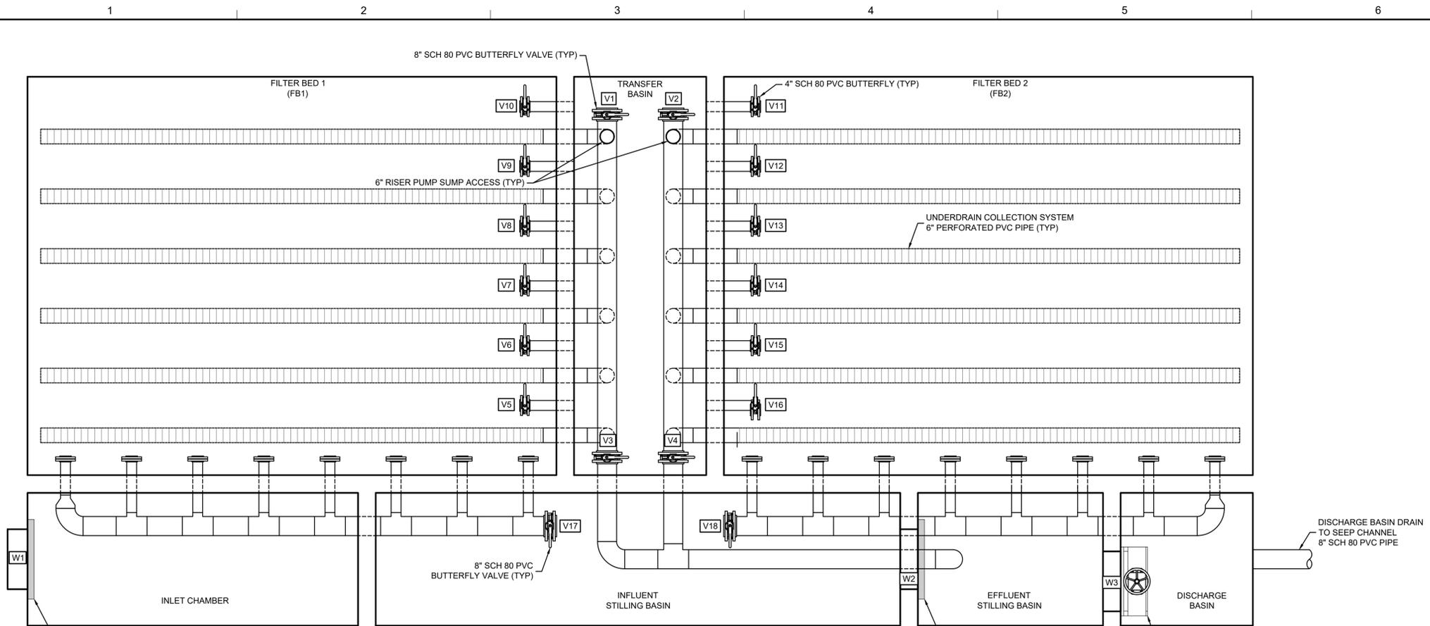
7 PLAN FLOW THROUGH CELL VALVE SCHEMATIC
